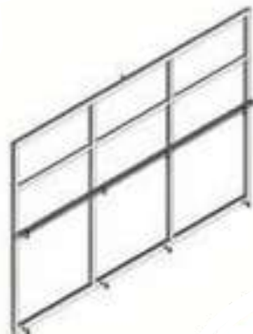
EXTENSION DE GARDE-CORPS
